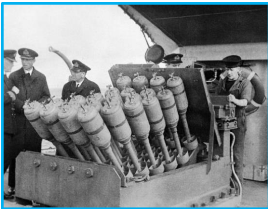
A Hedgehog anti-submarine mortar mounted on a ship
